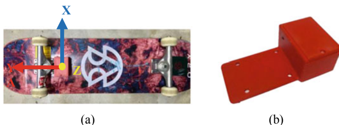
Fig. 2 The instrumented IMU attached at bottom front of the board, a Attachment of the IMU to the skateboard, b the 3D printed IMU device
