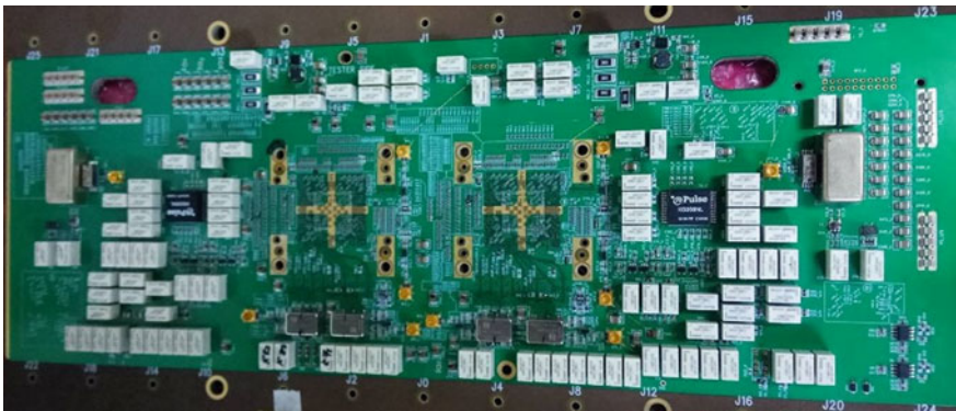
Fig. 1 Example of industrial PCB use in automated test equipment as a load board
