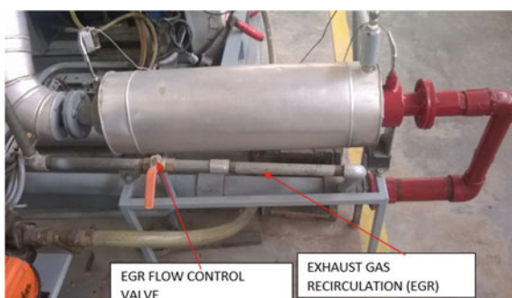
Fig. 4 Experimental exhaust gas recirculation (EGR) setup
