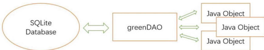
Fig. 1 Object relational mapping model diagram
