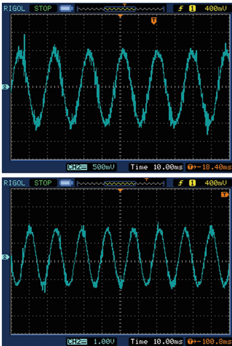
Fig. 4 Voltage waveform when the phase A on the inverter side outputs 50 and 35 Hz
