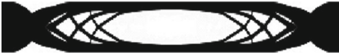
Fig. 4 Optimal topology of clamped beam with an optimized volume fraction of 0.6152 with natural frequency of 219.9838 rad/s for a specified frequency of 170 rad/s
