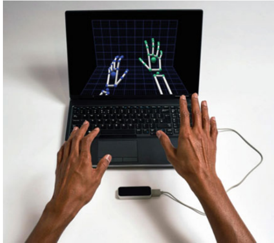
Fig. 7. Leap motion controller ( https://developer.leapmotion.com/ )
