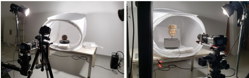
Fig. 2. Capturing setup in Museum of Islamic arts/media digital laboratory in Qatar
