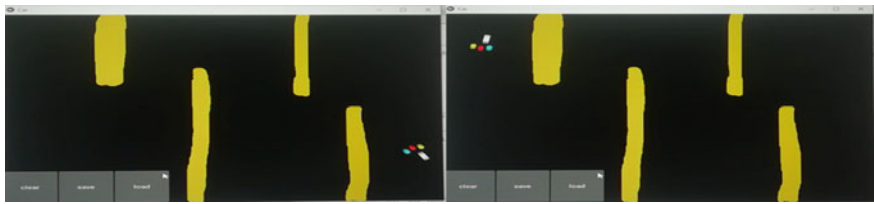
Fig. 5. Kivy platform with vehicle and sensors. Yellow curves denote obstacles. The vehicle moves from the bottom right corner to the top left corner
