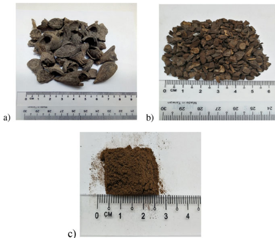
Fig. 1 Images of raw PKS a original form, b granulated form and c ground powder 250 \mu\text{m}
