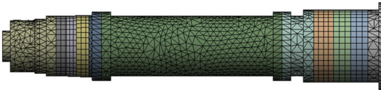
Fig. 7 Meshing of T385 turbine rotor-shaft model
