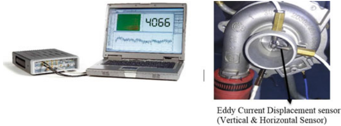
Fig. 8 Hardware and sensor instrumentation
