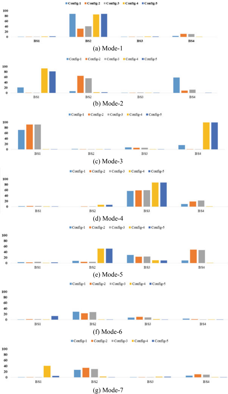
Fig. 4 % SE distribution in bearing supports for various configurations
