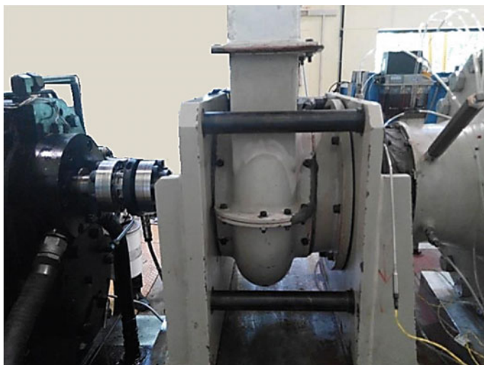
Fig. 15 Test section after instrumentation
