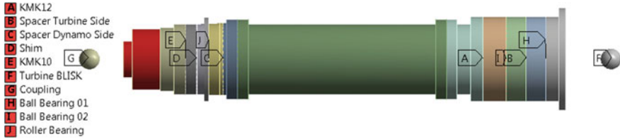
Fig. 6 T385 turbine rotor-shaft model with supported component locations
