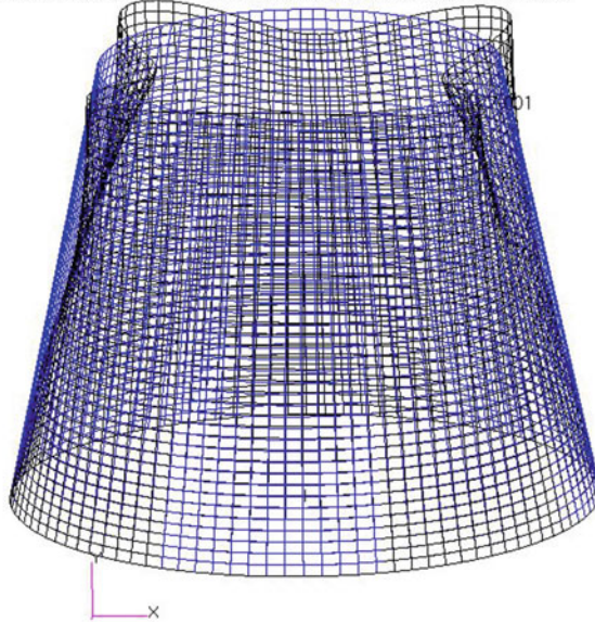
Fig. 11 First buckling mode of composite monocoque structure
