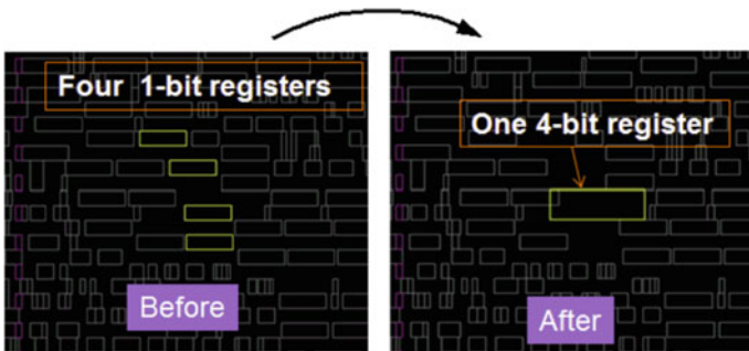
Fig. 6 Four 1-bit registers swapped into a single 4-bit register
