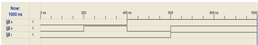
Fig. 17 Waveform of AND gate in Xilinx 8.1i
