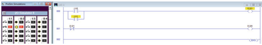
Fig. 12 NOR-gate implementation with input A = 0 and input B = 1 with auxiliary output = 1 and output Y = 0
