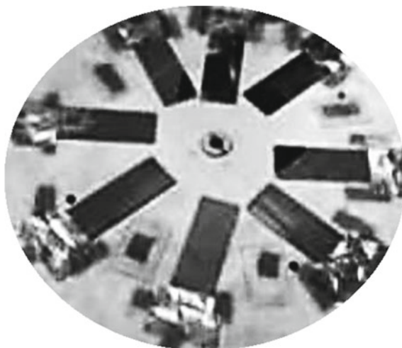
Fig. 2 Glass slides coated with the sandwich configuration of Al- \text{Sb}_2\text{Se}_3 -Al, where the two aluminum layers are 200 nm thick and the \text{Sb}_2\text{Se}_3 layer is 160 nm thick
