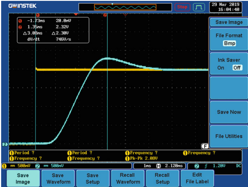
Fig. 5 Open-loop FSM output with an input of 0–2 V square wave of freq. 15 Hz, in finding t_p
