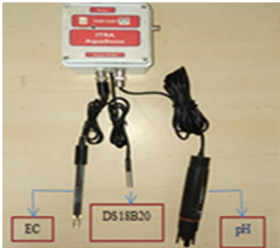
Fig. 12 Implementation of sensor node
