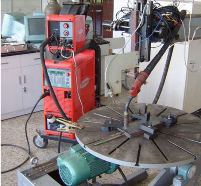
Fig. 4 DAQ system of arc sound signal in MIG welding
