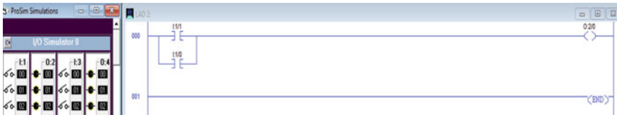
Fig. 6 OR-gate implementation with input A = 0 and input B = 0 with output Y = 0
