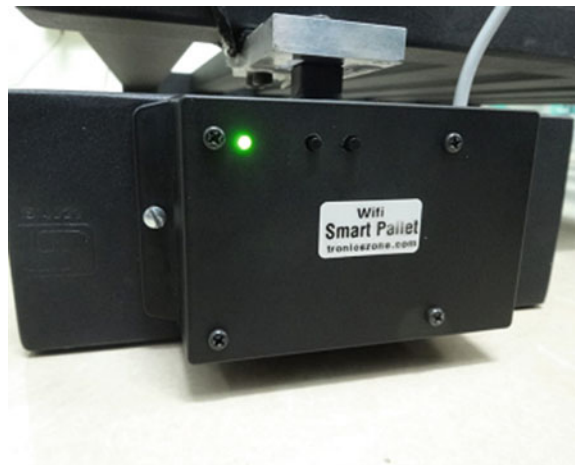
Fig. 3 WiFi smart pallet—WiFi weight sensor
