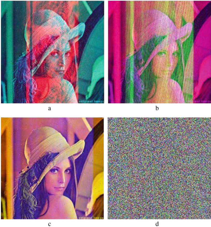
Fig. 5 Image decrypted using incorrect keys a when the fractional order of red is incorrect keeping all others same. Similarly for b green and c blue, d incorrect Arnold keys
