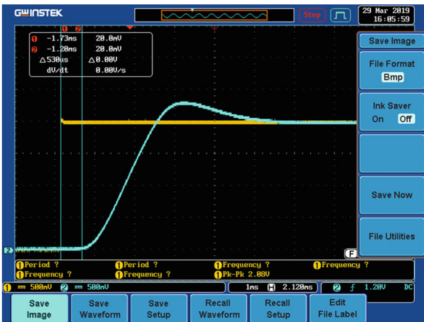
Fig. 4 Open-loop FSM output with an input of 0–2 V square wave of freq. 15 Hz, in finding t_d
