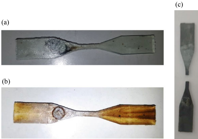
Fig. 2 Digital camera Images of Dog-bone shaped sample a Pure PC sample, b PC/Graphene (PCG) nanocomposites and c broken dog-bone sample after testing
