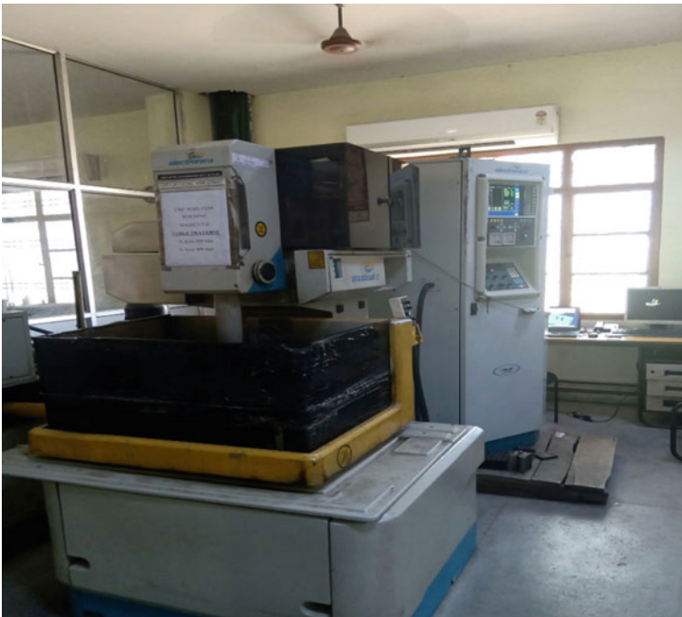
Fig. 1 WEDM machine set up
