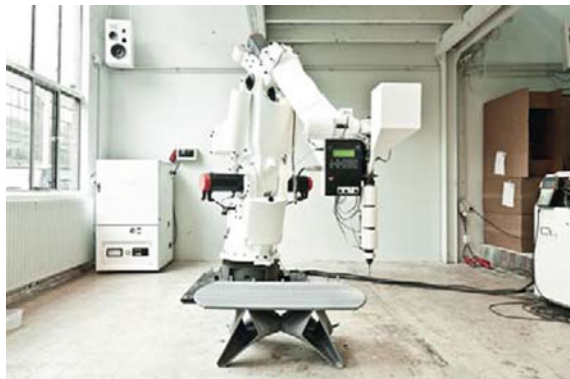
Fig. 2 Furoc 3D printer's robotic arms [6]. RFC of the waste sheet and then AM on the substrate by drop jet [30]
