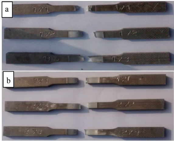
Fig. 10 Fractured Tensile specimens without interlayer
