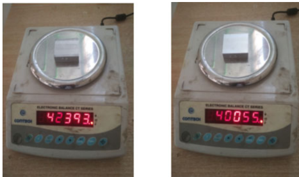
(a) Initial Weight (Before Machining) (b) Final Weight (After Machining)
