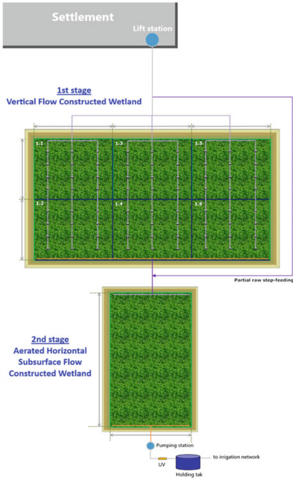
Fig. 7.1 A schematic representation of the treatment stages of the constructed wetland facility
