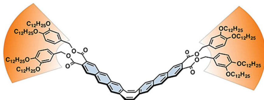
Fig. 20.6 Chemical structure of the light-melt adhesive. The orange moieties bring out the liquid crystal phase of the compound, the blue part causes photoreactions, and the central bent unit allows the molecules to move when exposed to light. The V-shaped molecular structure leads to a strong self-interaction (see Fig. 20.3) and realizes high cohesive force of the material
