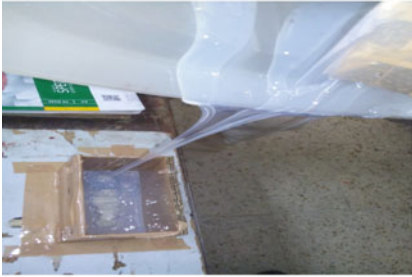
(c) Mixing rubber, hardener and pouring into the frame
