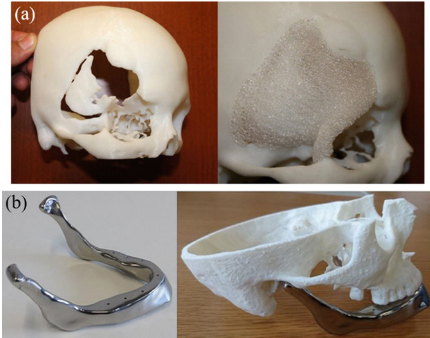
Fig. 6.4 a Skull model in ABS and PMMA placed in the cranial defect. Reproduced with permission from [70]. Copyright 2010, Emerald Publishing Limited. b Images of the post-processed mandibular implant and the representative FDM model in ABS of the skull/maxilla model with the final implant. Reproduced with permission from [72]. Copyright 2017, Knowledge E
