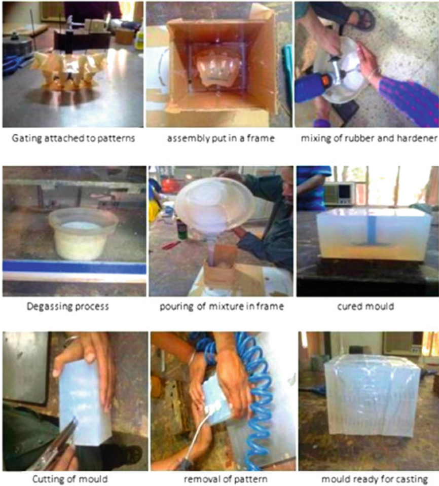
Fig. 7.11 Steps of preparing the silicon mould
