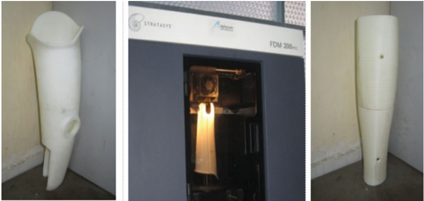
Fig. 12.8 Socket fabricate with FDM mc 200 machine
