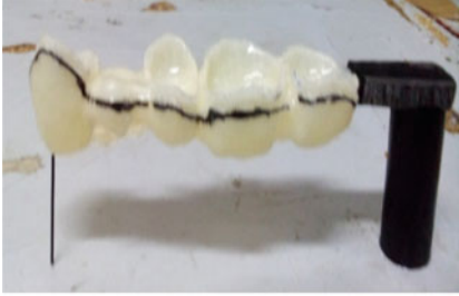
(a) Gate attached to FDM pattern
