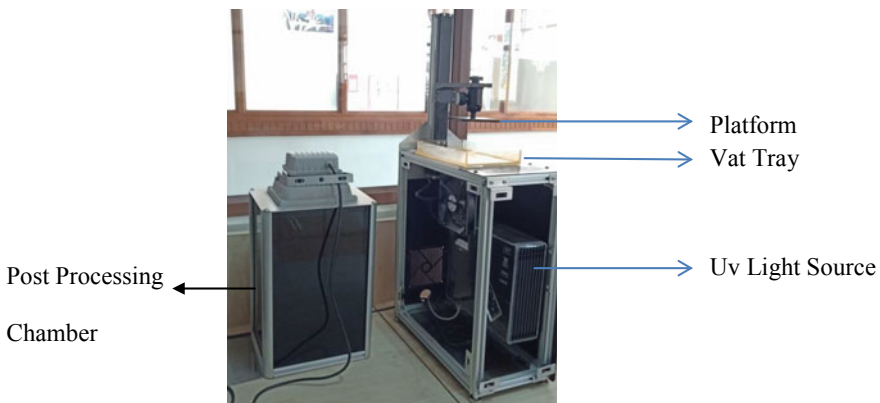
Fig. 9.3 Stereolithography KUDO 3D printing machine
