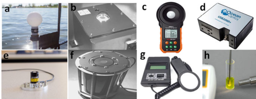
Fig. 2.1 Different types of light meters: the spherical photometers (a–c, h), planar lightmeter (e–g), and optical spectrum analyzer (d)
