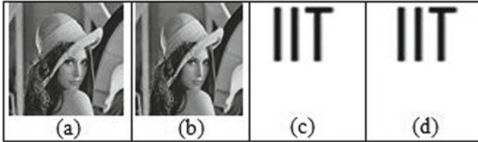
Fig. 5 a Original host Lena, b watermarked image (PSNR = 47.5923 dB), c watermark, d extracted watermark from unattacked watermarked image (NC = 0.9981)
