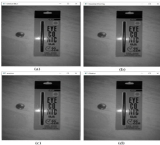
Fig. 3 Result of different preprocessing techniques (Parenthesis) a Result of median blur, b Result of Gaussian blur, c Result of erosion, and d Result of Dilation
