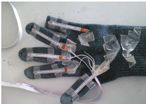
Fig. 7 Data glove with flex sensors
