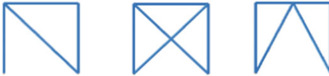
Fig. 2 Types of braces used are, diagonal brace, cross (X) brace and chevron brace, from left to right
