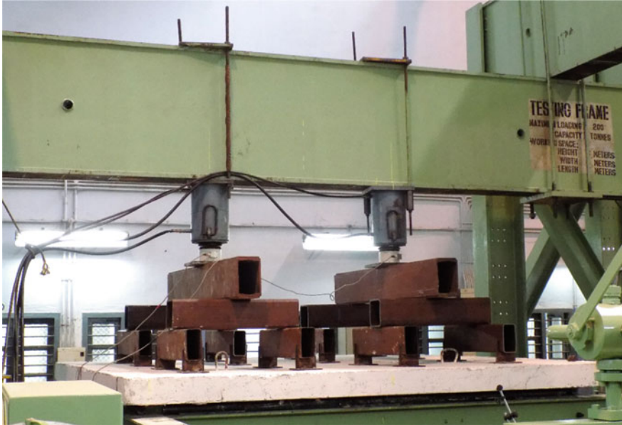
Fig. 4 Two-way flexural test set-up (16-point load)
