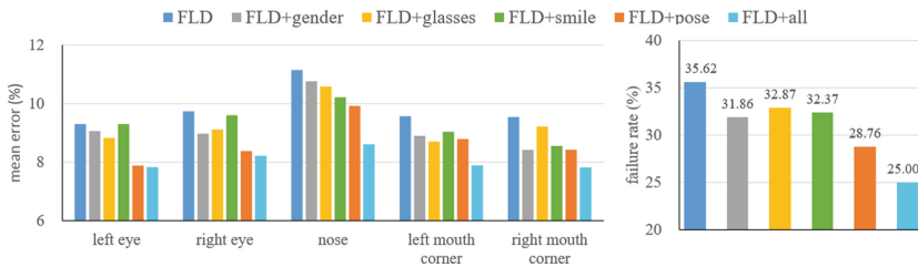
Fig. 3. Comparison of different model variants: the mean error over different landmarks, and the overall failure rate [5].
