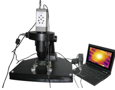
Fig. 1. Laboratory new thermal imaging system
