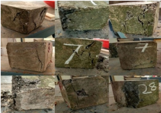
Fig. 7 Failure pattern of HPC cube
