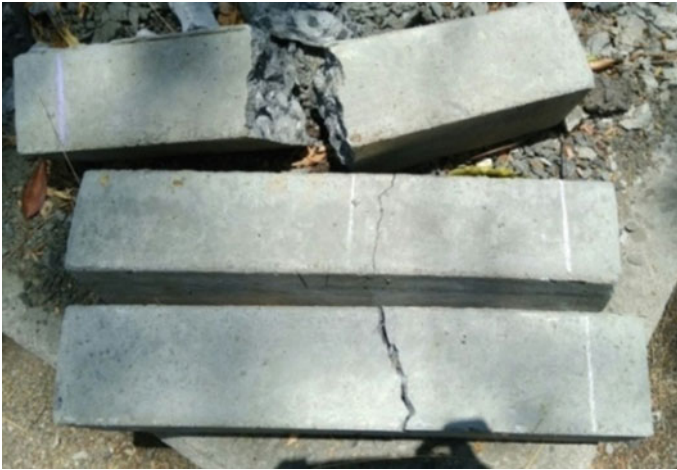
Fig. 8 Failure pattern of the prism of M20 grade concrete
