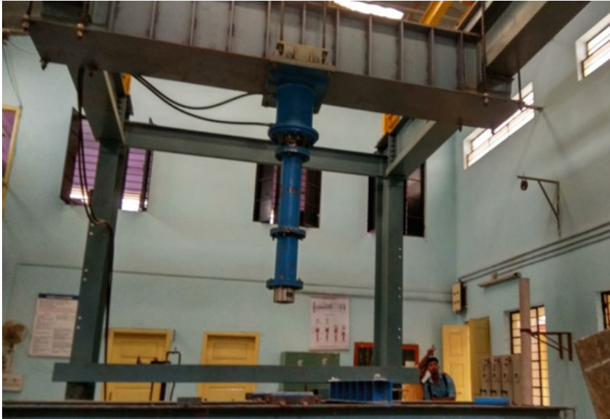
Fig. 4 Testing arrangement for RC beams
