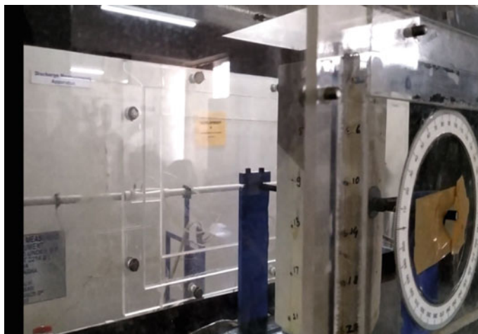
Fig. 13 Drag for hexagonal shape by wind tunnel
