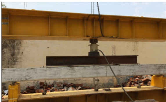
Fig. 2 Test setup for testing the beams
