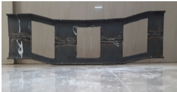
Fig. 7 Web and flange buckling is observed in the beam with rectangular opening CSBIR 1
