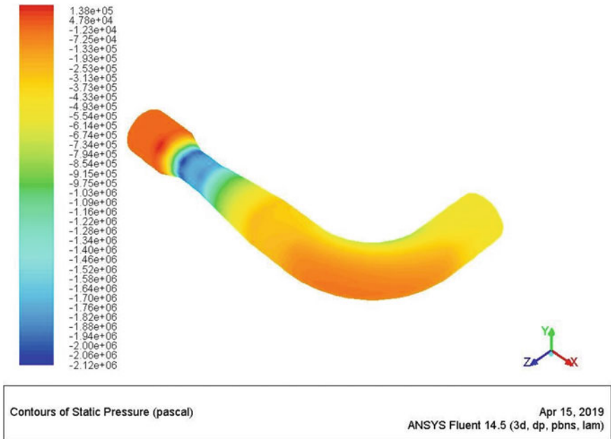
Fig. 8 Contours of Static pressure with pipe bend
