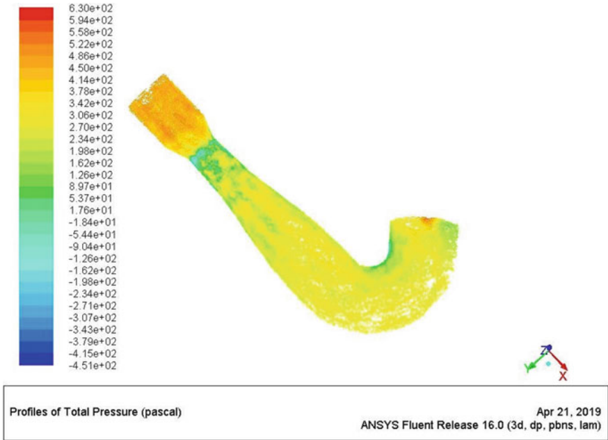
Fig. 13 Venturimeter with an acute bend
