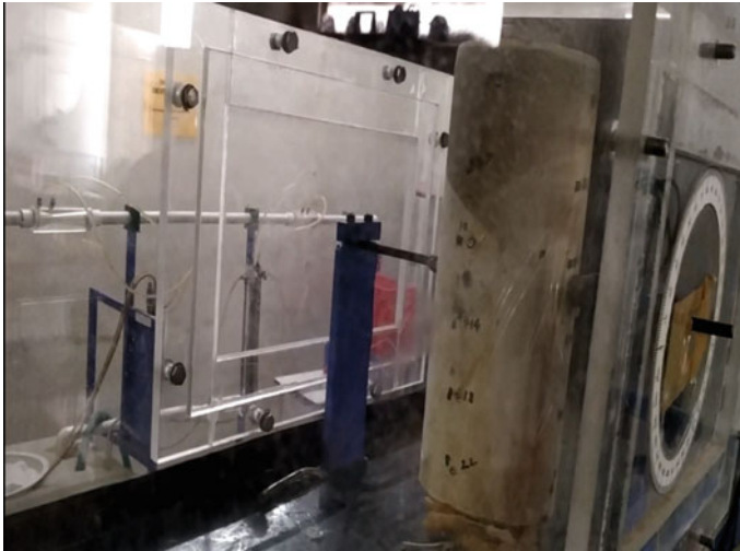
Fig. 10 Drag coefficient for circular shape by wind tunnel
