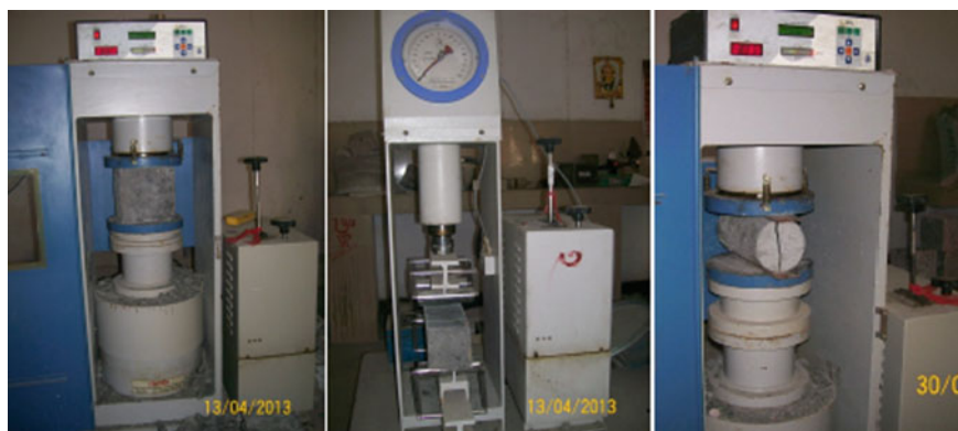
Fig. 2 Arrangement for compressive, flexural and split tensile strength
