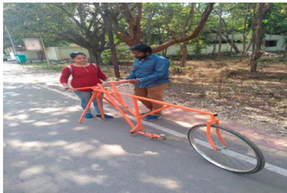
Fig. 5 Merlin equipment while working (author Mandeep Kaur Arora along with co-author Mahesh Ram Patel recording data)
