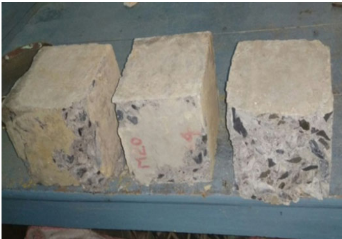
Fig. 6 Failure pattern of cube M20 grade
