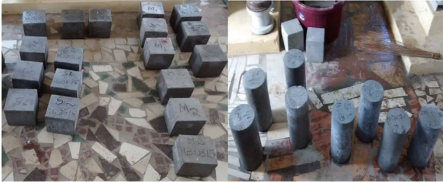
Fig. 2 Cubes and cylinders after 28 days of curing
