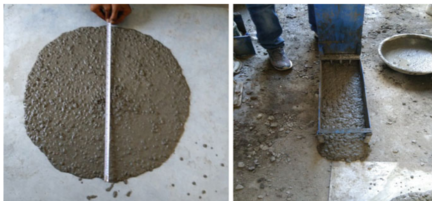
Fig. 6 Slump flow test and L-Box test of SCC
