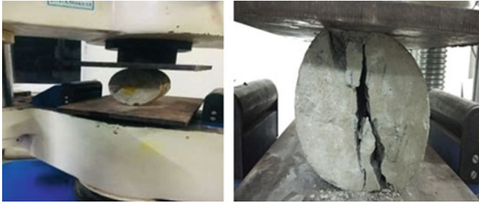
Fig. 7 Tensile test for sample prepared
