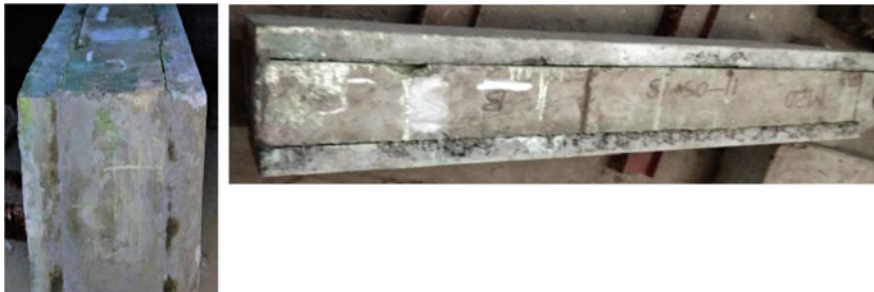
Fig. 2 Beam with HPC U-shape jacket (top view and side view)
