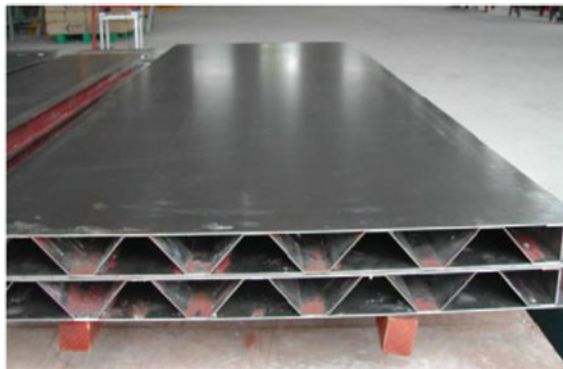
Fig. 9 Double-skin steel panel. (Source Hong et al. [14])
