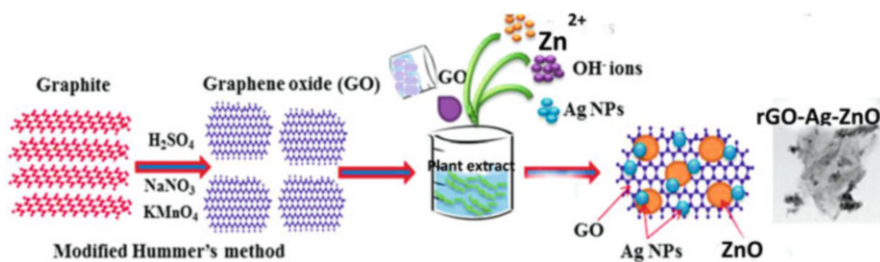
Fig. 2.10 Green synthetic pathway for preparation of rGO-Ag-ZnO nanocomposites
