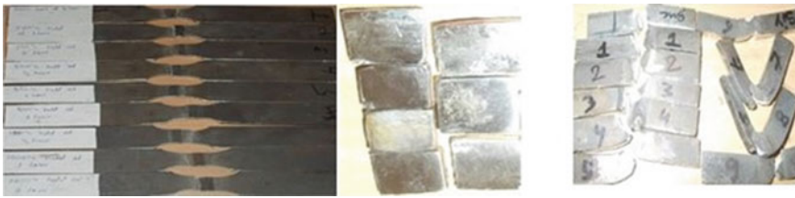
Fig. 3 Tensile-, microhardness-, and impact-tested specimens viewing the place of fracture at different normalization temperature
