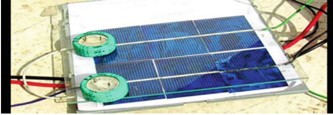
Fig. 6 Super capacitor technology to reduce the partial shading affects
