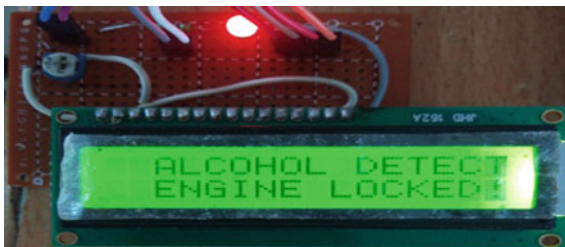
Fig. 9 Status of LCD when alcohol detection
