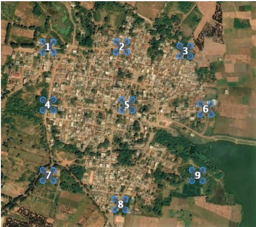
Fig. 1 Arrangement of the UAVS over the village to form a cluster
