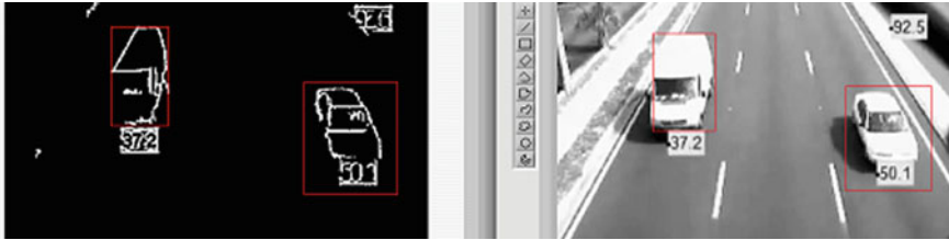
Fig. 4 Detection and counting of cars after application of background subtraction
