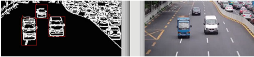
Fig. 3 Detected cars after application of edge threshold algorithm
