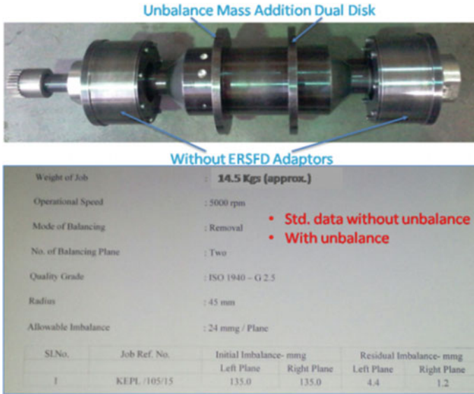
Fig. 12 Dynamic balancing of rotor
