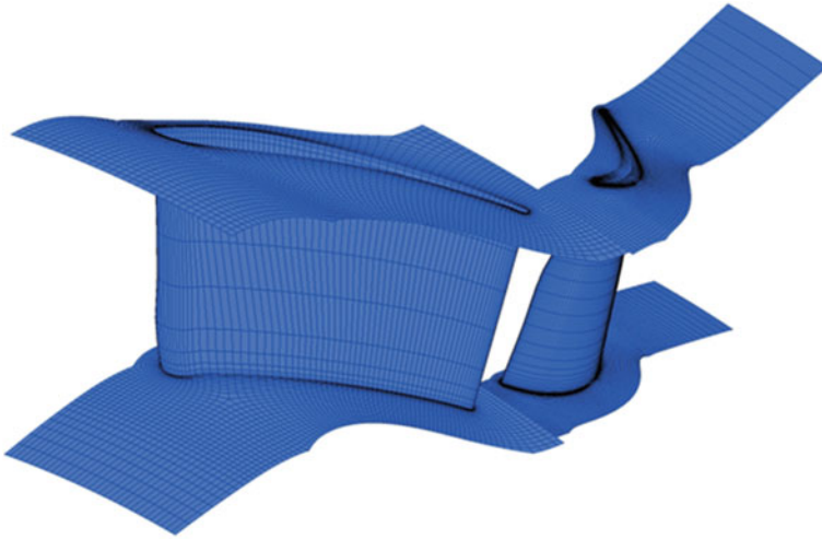
Fig. 1 HP turbine computational grid
