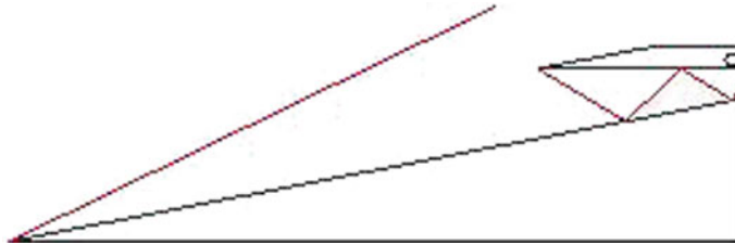
Fig. 4 Shock reflection configuration in the inlet when the Freestream Mach number is below the design Mach number
