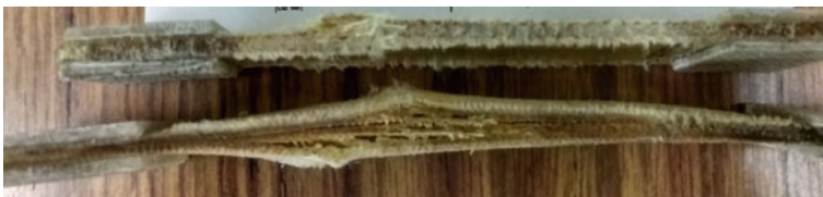
Fig. 5 Change in failure modes in multilayer-composite specimens with fiber orientation
