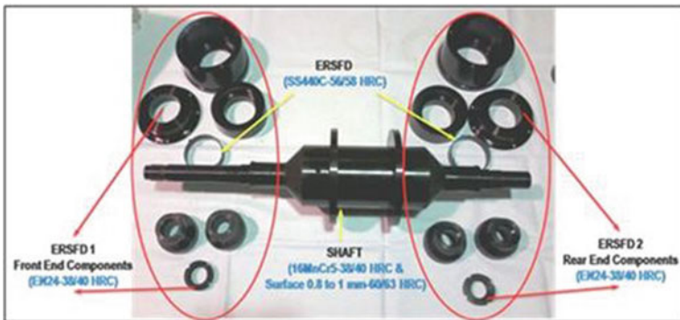
Fig. 11 ERSFD test rig and rotor system components
