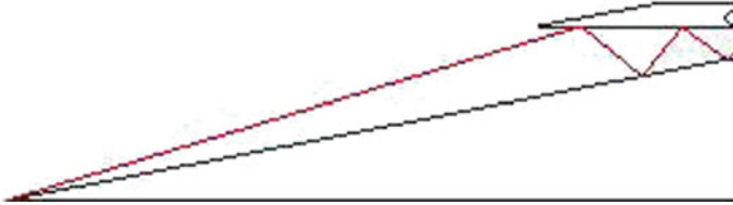
Fig. 3 Shock reflection configuration in the inlet when the Freestream Mach no. is above the design Mach no
