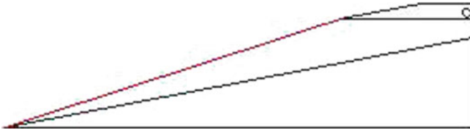
Fig. 2 Inlet operation at design Mach number (shock on lip condition)
