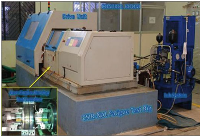
Fig. 10 Aero-engine bearing fatigue test rig for ERSFD testing
