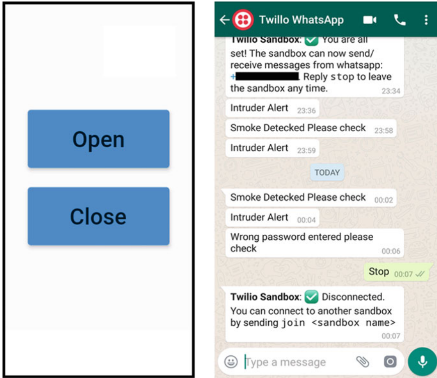
Fig. 8 Mobile application and WhatsApp alert feature of the system
