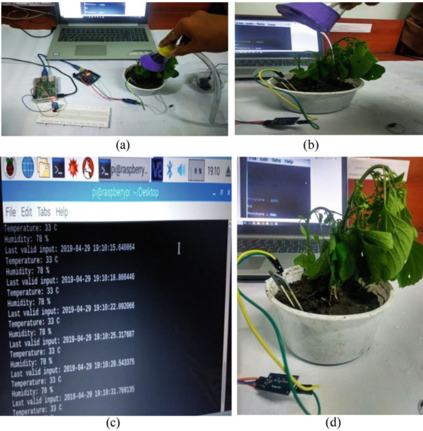
Fig. 4 a Real-time setup of the Raspberry pi. b Automatic water sprinkler connected immersed pump. c Real-time temperature and humidity data acquired in Pi. d Test set up
