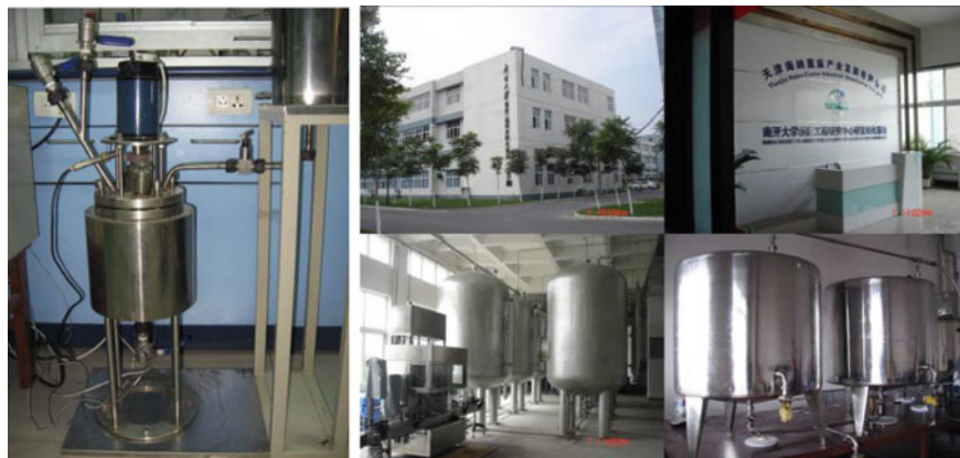
Fig. 7.7 Bench scale facility for sebacic acid preparation (left) and Pilot plant for production of environmentally friendly castor-based lubricate with annual capacity of 5000 tons (right)
