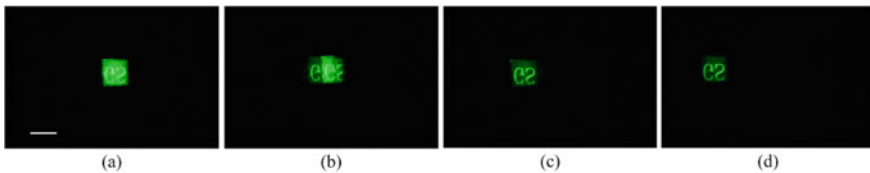
Fig. 12.8 Holographic reconstructions in the image plane without undesired orders, scale bar is 6.0 mm, a basic 4f setup, b 8 pixels per period, c 4 pixels per period, d 2 pixels per period
