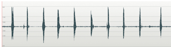
Fig. 3. Time domain representation of the audio file consisting of the utterance of one speaker speaking digits 0 through 9
