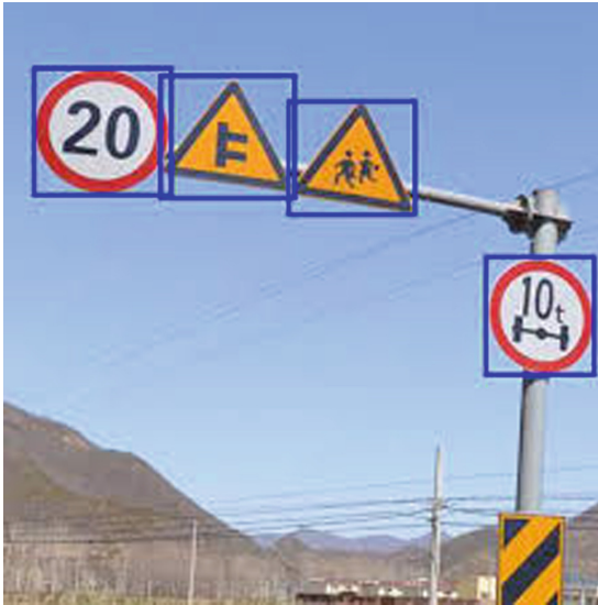
Fig. 1. Detection of sign boards as individual objects from image
