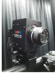
Fig. 6. Multispectral camera “FluxData FD-1665 (USA).”
