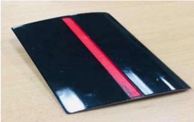
Fig. 1 The NACA 4415 airfoil with slot for vortex generator at 50%C
