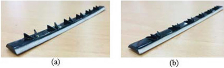
Fig. 2 (a) Triangular counter-rotating vortex generator, (b) shark skin shape counter-rotating vortex generator
