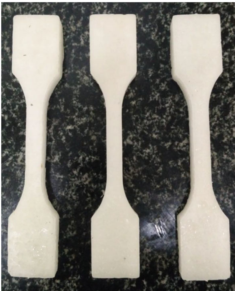
Fig. 1 Macrostructure of 80P fuel samples obtained from dog bone shape die
