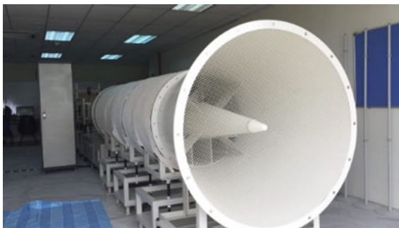
Fig. 6 Subsonic wind tunnel
