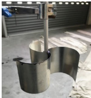
Fig. 3 The 3-bladed Savonius hydrokinetic turbine model
