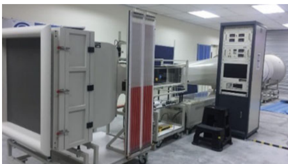
Fig. 7 Control system and test section of wind tunnel
