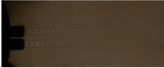
Fig. 7 Shadowgraph picture of circle-circle twin jet at NPR 2
