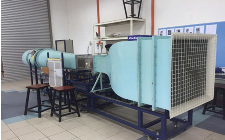
Fig. 4 Open circuit subsonic wind tunnel for the NACA 4415 airfoils test
