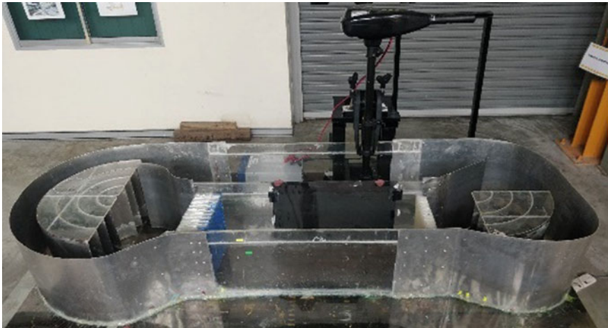
Fig. 3 Fabricated Modified Water Tunnel
