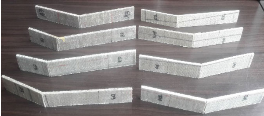
Fig. 5 Tensile properties tested samples of treated and untreated biotex flax fiber-reinforced composite
