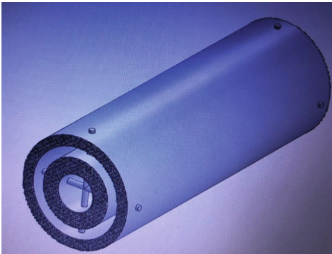
Fig. 2 Two layer desiccant bed
