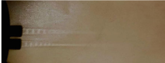
Fig. 8 Shadowgraph picture of circle-ellipse twin jet at NPR 2
