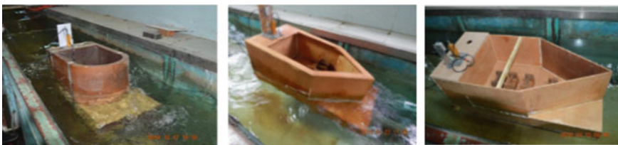
Fig. 7 The models for Model A, Model B, and Model C [26]
