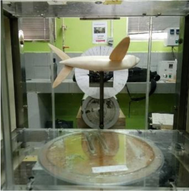
Fig. 3 Exocoetus Volitans model in the test section of the wind tunnel
