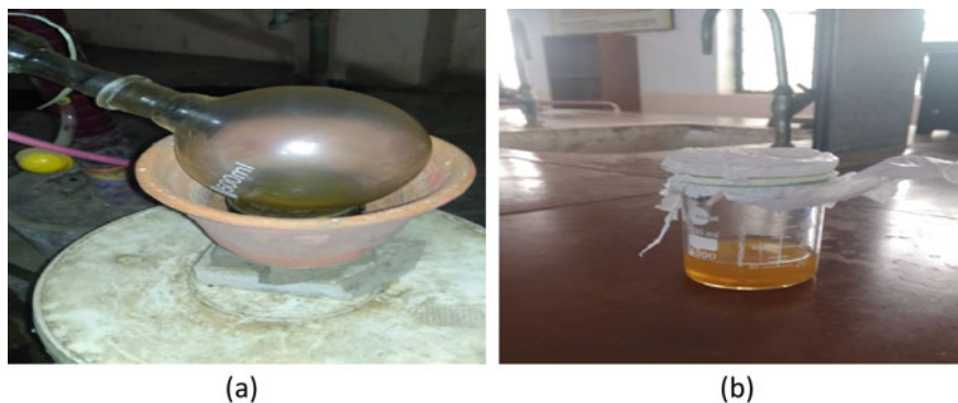
Fig. 4 a Fuel getting collected in the RB flask, b Fuel collected at the end of the experiment
