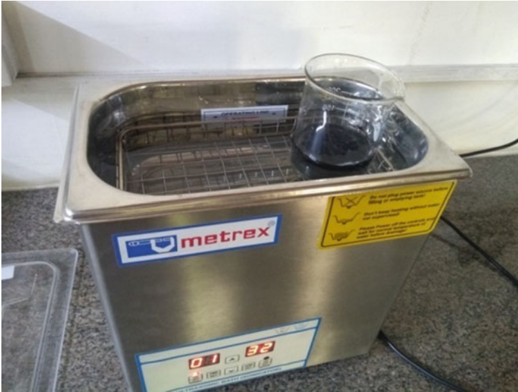
Fig. 5 Sonication of graphene oxide solution
