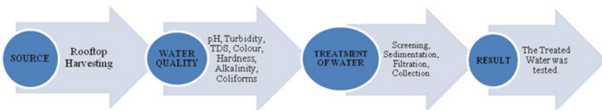
Fig. 2 Block diagram with all included steps for surface runoff treatment to access as per usability
