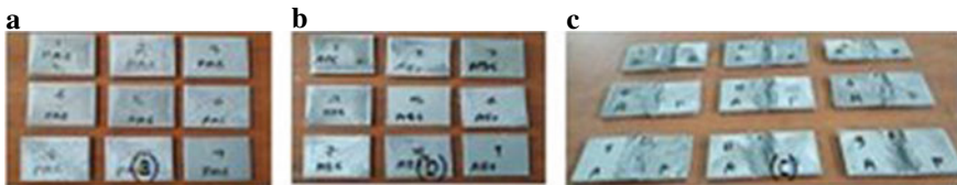
Fig. 2 3D printed parts of a PA6-50%Al, b ABS-15%Al and c joints by FSW process
