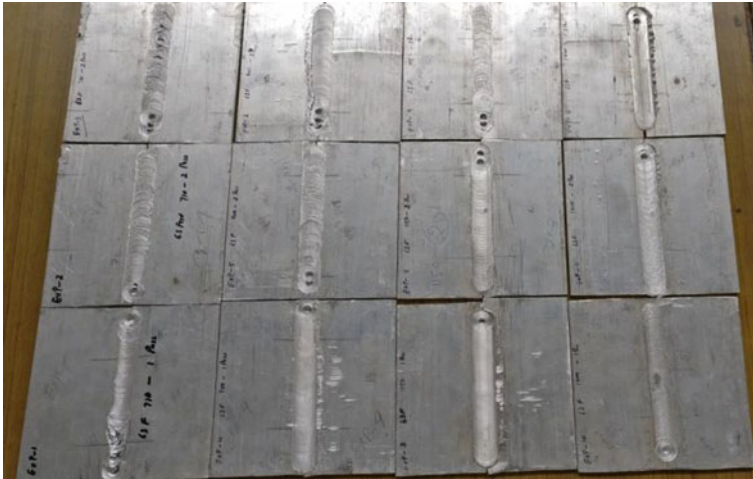
Fig. 3 FSWed joints of AA6082-T6 aluminum alloy
