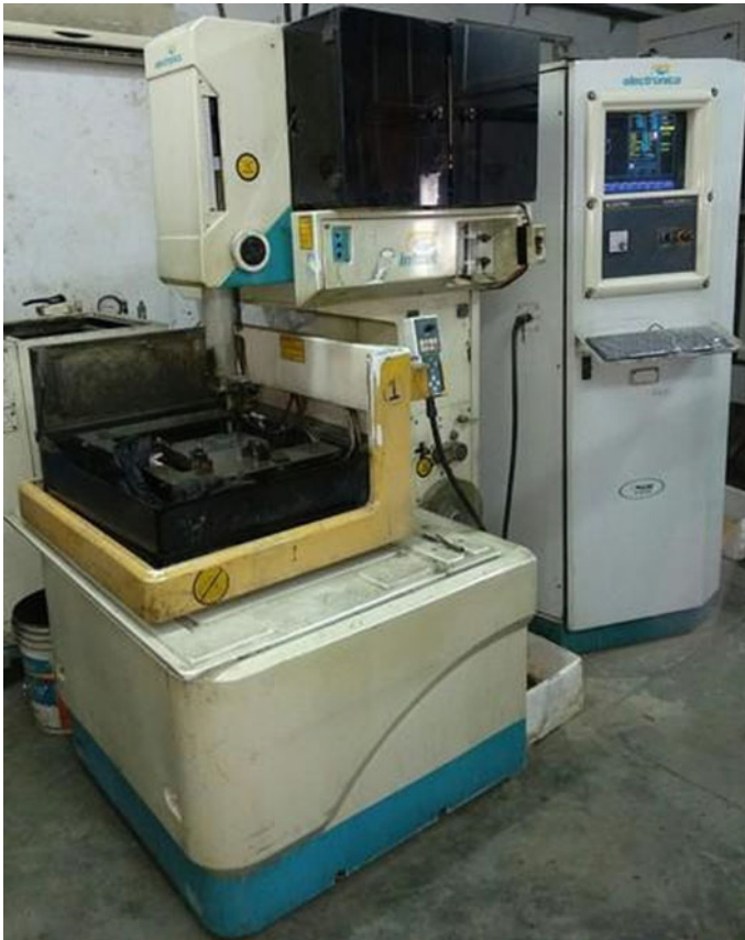
Fig. 1 Schematic representation of WEDM machine
