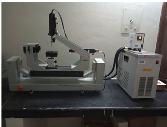
Fig. 6 Drop shape analyzer measuring the water contact angle
