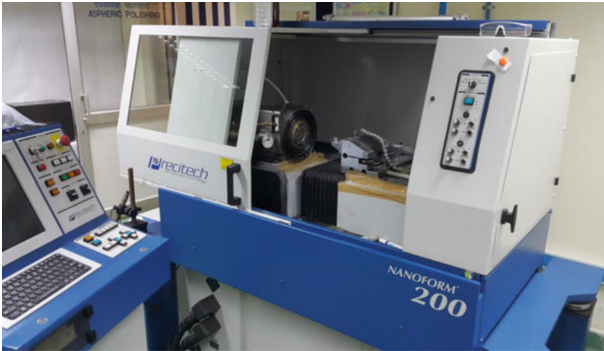
Fig. 1 Nanoform-200, Single Point Diamond Turning (SPDT) machine
