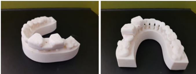
Fig. 9 3D printed drill guide
