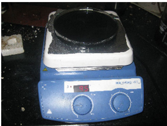
Fig. 8 Homogeneous composite solution placed on a hot plate for evaporation process
