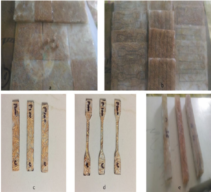
Fig. 2 a. Workpieces after taking from the glass moulds. b. Workpieces in the glass moulds after taking out of furnace. c, d, e. Testing samples
