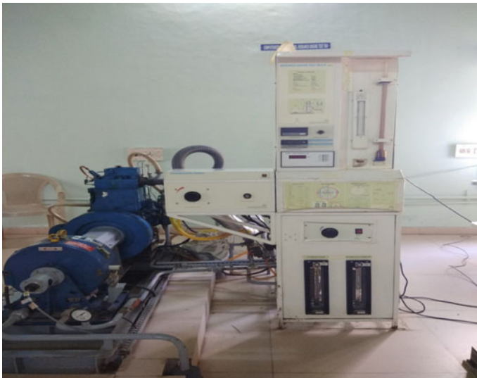
Fig. 2 Experimental setup of CI engine
