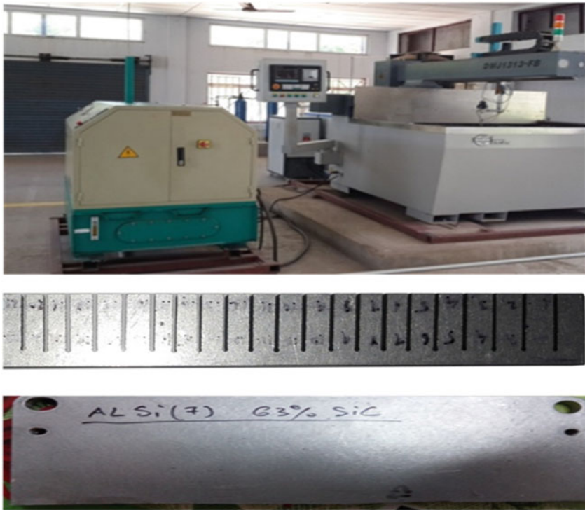
Fig. 1 Abrasive water jet machine and the test sample
