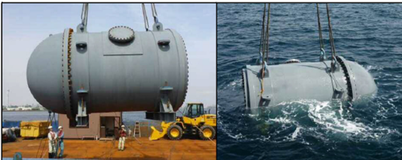
Fig. 5. Pressure test with using mock-up model
