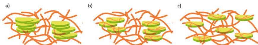
Fig. 4 Clay–polymer interactions: a polymer/clay blend, b polymer/clay intercalation, c exfoliation of clay in polymer matrix
