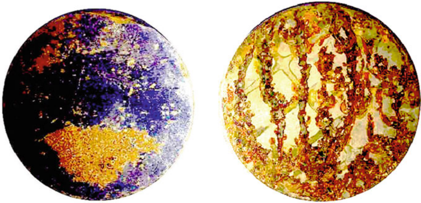
Fig. 26.1 Salt spray tested specimen in 5% NaCl after 24 h in spray chamber WHT specimen on left and HT specimen on the right
