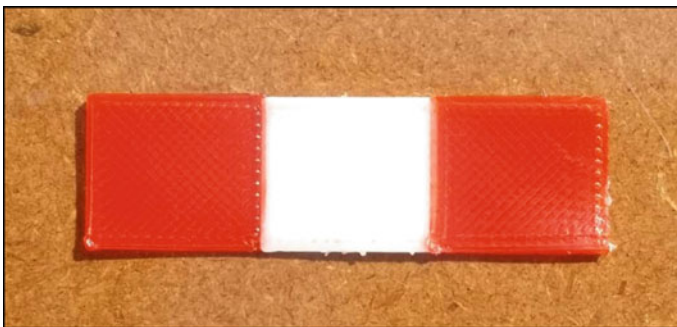
Fig. 3.2 Fabricated part joins with dissimilar material
