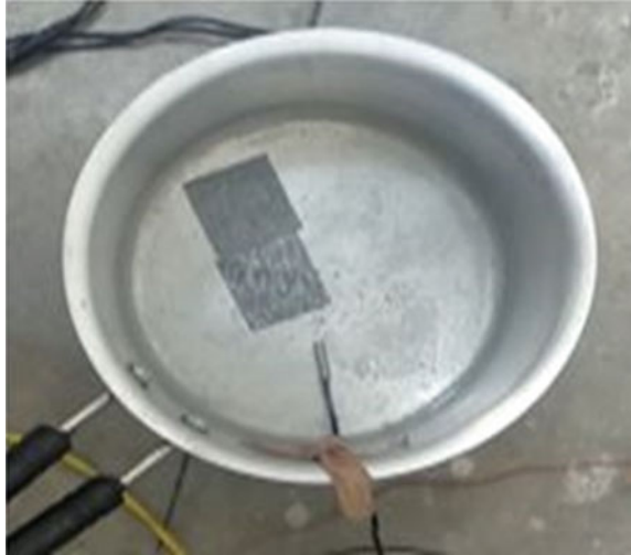
Fig. 6.7 Boiling of etched samples by immersing in water
