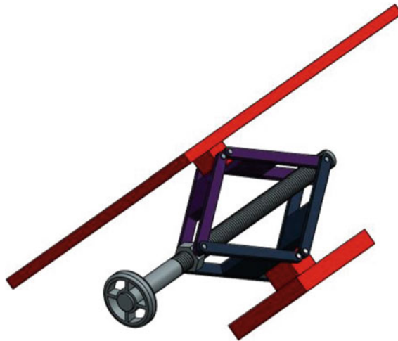
Fig. 11.20 Screw jack for providing vertical lifting of welding torch assembly
