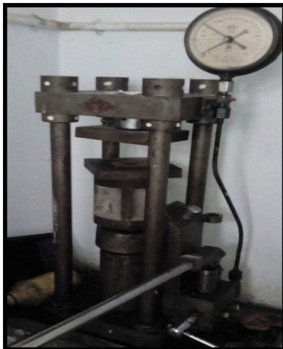
Fig. 27.1 Hydraulic compaction machine (specification-maximum load = 250 KN, ram diameter = 75 mm, AMIL India, S. No. 86019, IITBHU)
