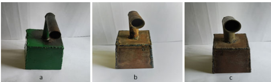
Fig. 4.3 Pouring sprouts of different sprue diameter
