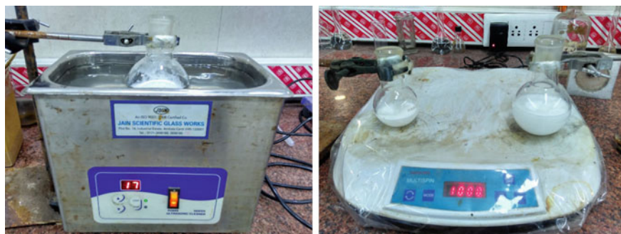
Fig. 8.4 Solution preparation for dip coating a Sonication for 20 min and b magnetically stirred for 30 min
