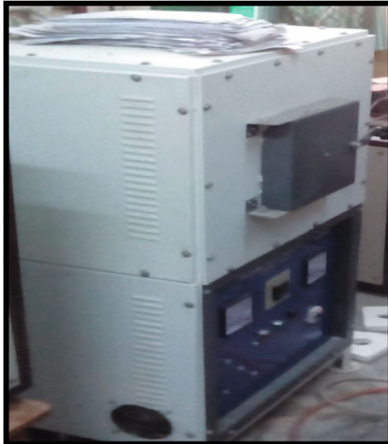
Fig. 27.2 High-temperature muffle furnace (maximum temperature of 1450 °C, 0–100 Amp, 0–150 V SISCO India, IITBHU)
