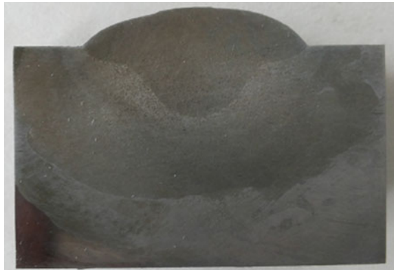
Fig. 25.1 For weld number 11, revealed bead geometry after etching
