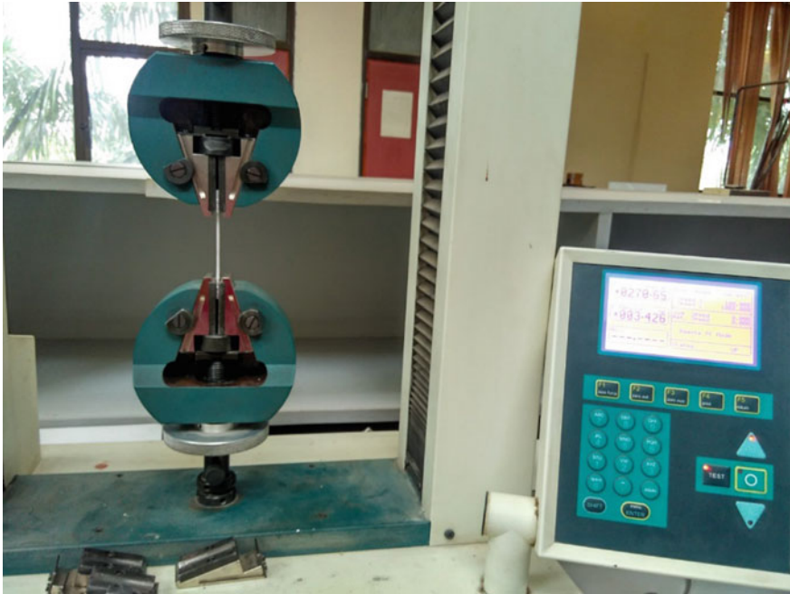
Fig. 3.6 Tinius Olsen H25KS universal tensile testing machine
