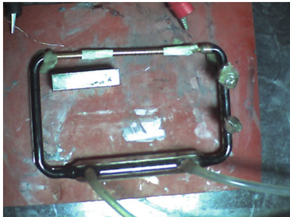
Fig. 44.3 Ferrofluid-based cooling system experimental setup
