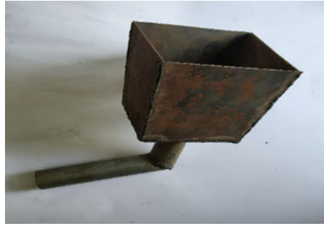
Fig. 4.4 Actual view of pouring spout
