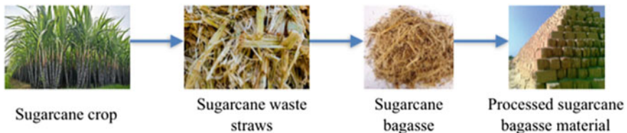
Fig. 32.7 Sequence of stages involved in getting processed sugarcane bagasse material from raw sugarcane crop
