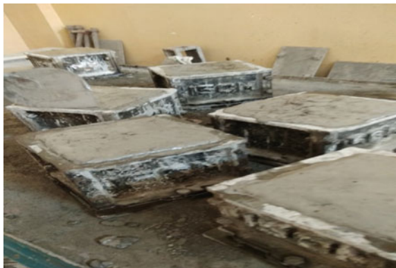
Fig. 6 Cubes compaction by vibrating table
