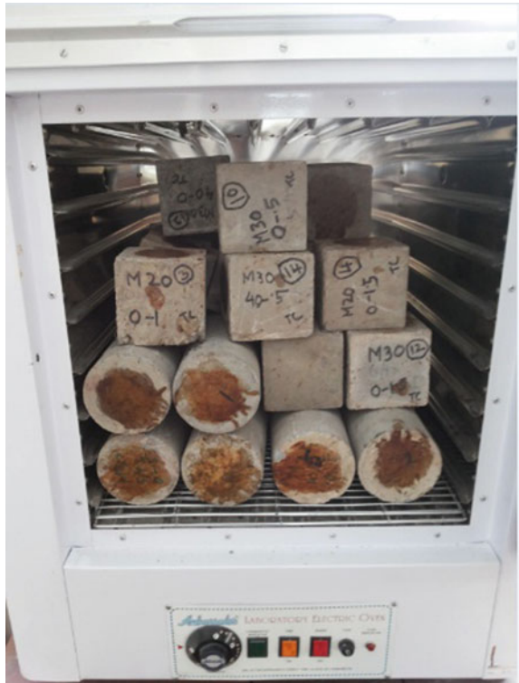
Fig. 5 Concrete specimens subjected to elevated temperature
