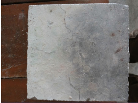
Fig. 9 Concrete specimens after exposed to 600 °C temperature
