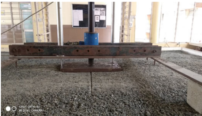
Fig. 4 Load-bearing test on rectangular footing
