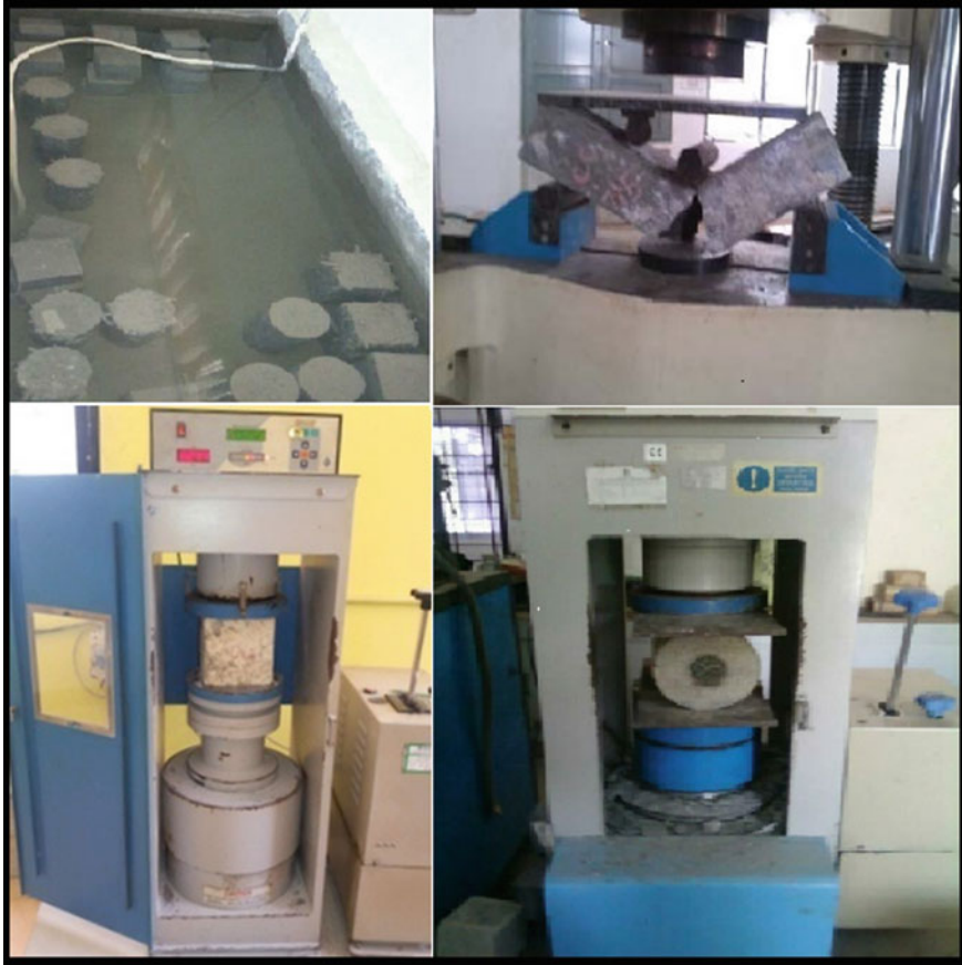
Fig. 2 Curing and testing of concrete specimens
