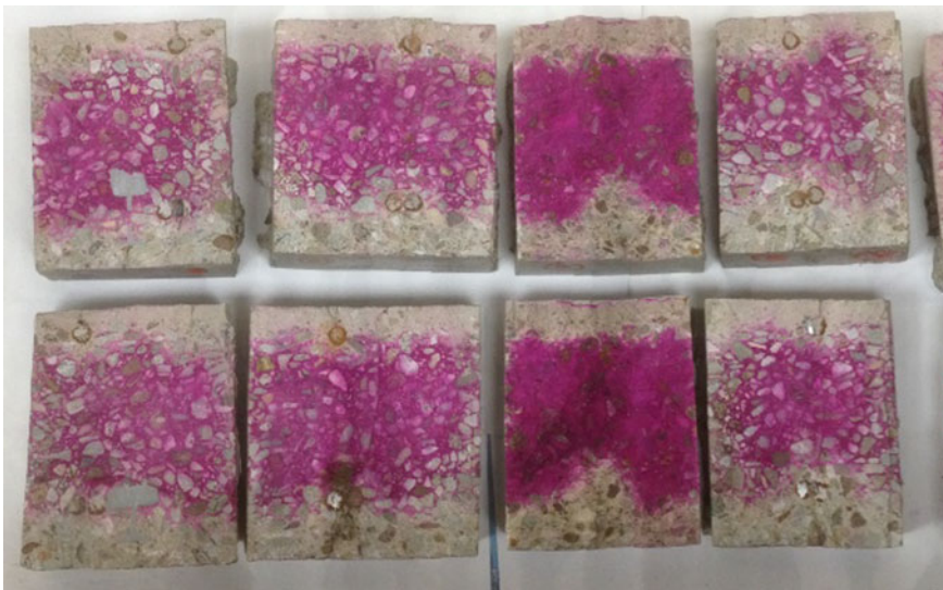
Fig. 6 Cube specimen are not affected by carbonation
