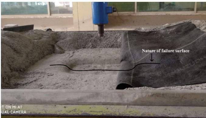
Fig. 7 Nature of failure surface below footing
