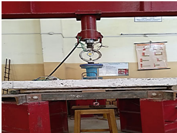
Fig. 7 Test setup with slab
