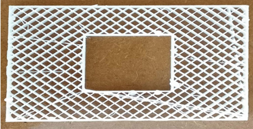
Fig. 9.2 Part made with faulty algorithm
