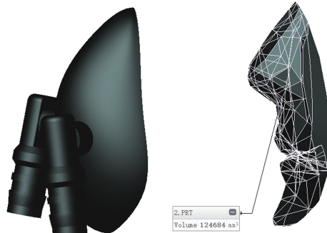
Fig. 10. The volume of the patient’s face, mouth and nose entering the oxygen mask model (after)
