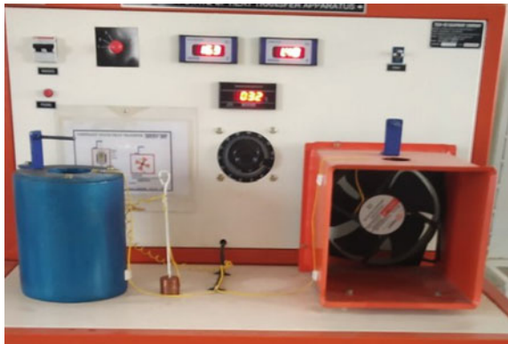
Fig. 6 Unsteady state heat transfer apparatus
