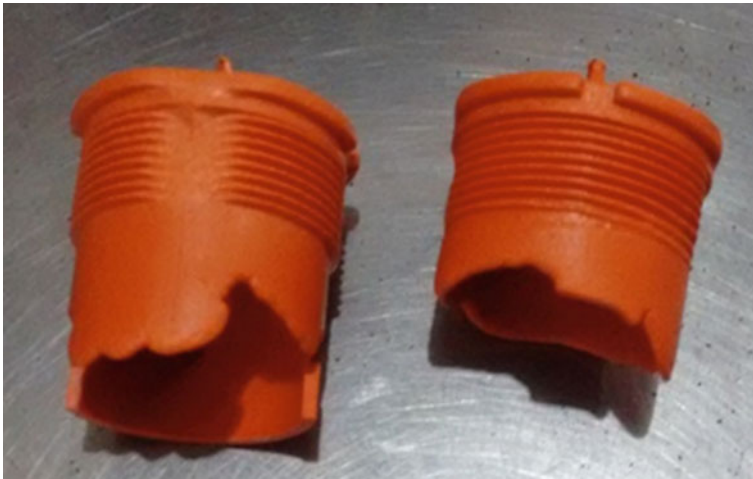
Fig. 2 Component with short shot-type defect
