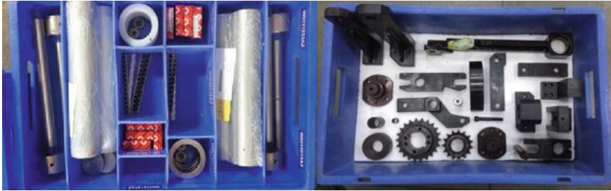
Fig. 3 Left: kit containing separate racks for parts as well as drawings and right: Poka-yoke implemented in the kit to avoid the mistakes while filling of the kits
