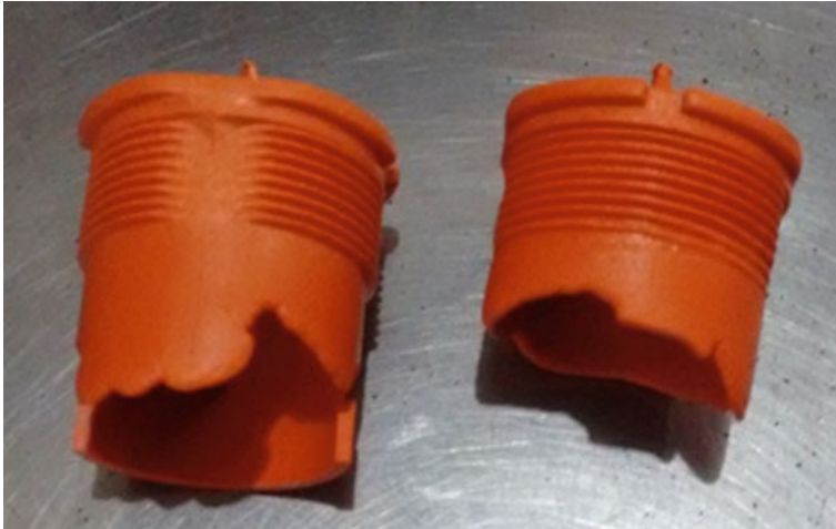
Fig. 2 Component with short shot-type defect
