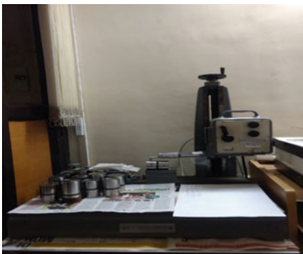
Fig. 1 Talysurf4 surface roughness measuring machine and surface roughness profile
