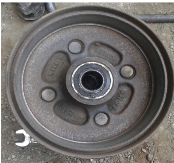
Fig. 2 Used drum for microstructure and Ra value
