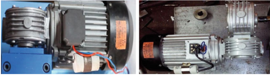
Fig. 2 This figure shows the constructional details of the primary motor (on left side) and secondary motor (on right side)
