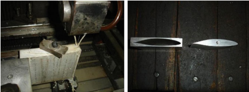
Fig. 26 The plain model of the aerofoil (by Wirecut M/C)
