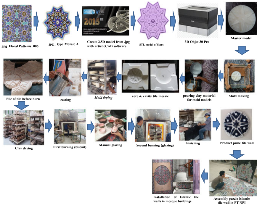
Fig. 8 General stages of CARESystem application in the phase of design, manufacturing, and fabrication of ceramic wall in the local Indonesian ceramic industry
