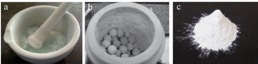
Fig. 1 Glass powder (GP) refining process. a Collision with mortar and pestle, b fineness by milling method [7], c the result of fine glass powder
