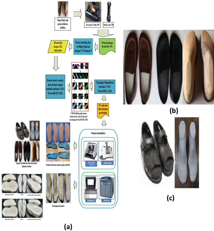
Fig. 4 a Architectural design and manufacturing shoes CARESystem based AFO. b Footwear AFO type 1. c Footwear AFO type 2
