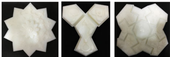
Fig. 3 The ceramic tile mold pattern master output from 3D print objet 30 Pro
