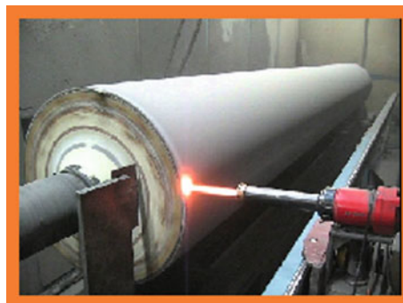
Fig. 8.3 Self-fluxing alloys/Ni-Cr-B-Si: used at shafts, sleeves due to its high hardness, almost no pores after fusing [38]
